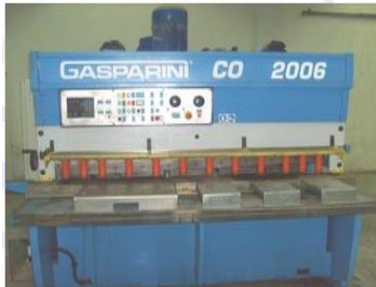
Figure 4. Shear cutting machine
